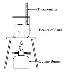
(a) Calculate the amount of heat energy needed to raise the temperature of the beaker of sand by 180.°C. Assume that all the heat energy from the burner is transferred to the beaker of sand and that the specific heat capacity of the beaker and sand together is 0.810 J/(g·°C).
